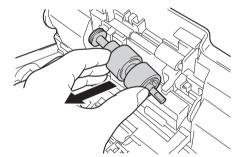
4 Remove the old Reverse Roller from the shaft and insert the new Reverse Roller all the way onto the shaft.
