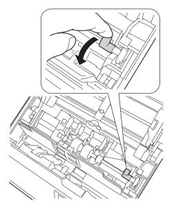
12 Pinch the Separation Roller and pull it out of the machine.
