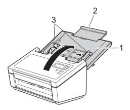
2 Pull the Output Tray (1) out of the machine and then unfold the Document Stopper (2).
