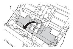
8 Pinch the Pick-up Roller and pull it out of the machine.
