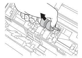
9 Pull the blue hook on the Separation Roller down.
