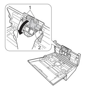
5 Pinch the Reverse Roller and pull it out of the machine.
