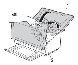
3 In the ADF unit, clean the glass strips (1) and feed rollers (2) with a soft lint-free cloth moistened with water.
