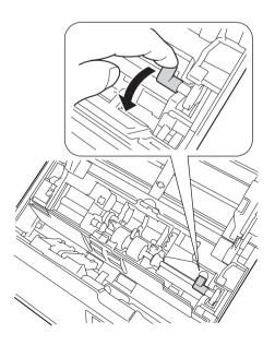
10 Pinch the Separation Roller and pull it out of the machine.
