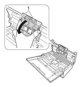
3 Pinch the Reverse Roller and pull it out of the machine.
