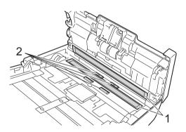
4 Press and hold the buttons (1) on the inside of the ADF Cover and then pull the Reverse Roller Cover (2) down.
