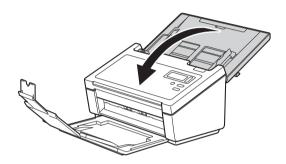
Close and push the Output Tray firmly back into the machine.
