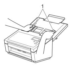
3 Set the Carrier Sheet in the ADF between the Guides until you feel it touch the inside of the machine.
