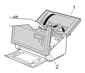
2 Press and hold the buttons (1) on the inside of the ADF Cover and then pull the Reverse Roller Cover (2) down.
