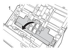
10 Pinch the Pick-up Roller and pull it out of the machine.
